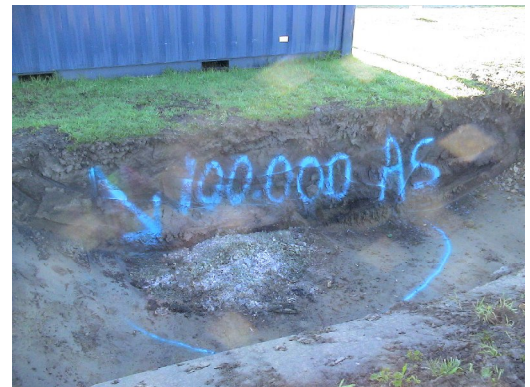
Figure 5 A quick XRF check revealed extreme copper, chromium & arsenic concentrations
